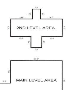
1 = 18 Scale: AREA CALCULATIONS SUMMARY BUILDING AREA BREAKDOWN Code Description Size **Net Totals** Breakdown Subtotals MAIN LEVEL AREA 1228.30 GBA1 MAIN LEVEL AREA 2ND LEVEL AREA 4.0 x 604.70 1833.00 8.2 32.80 8.0 ж 12.9 103.20 33.0 x 33.1 1092.30 2ND LEVEL AREA 5.0 x 7.0 × 67.20 33.0 495.00 TOTAL BUILDING 1833 6 Calculations Total (rounded) (rounded) 1833
